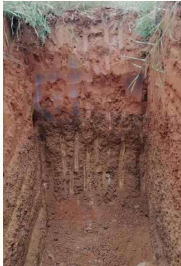
Figure 2: Typical profile, hardpan ferricrete (left) underlain by collapsible residual granite (right)
