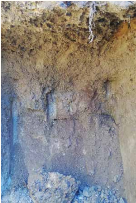
Figure 2: Typical profile, hardpan ferricrete (left) underlain by collapsible residual granite (right)
