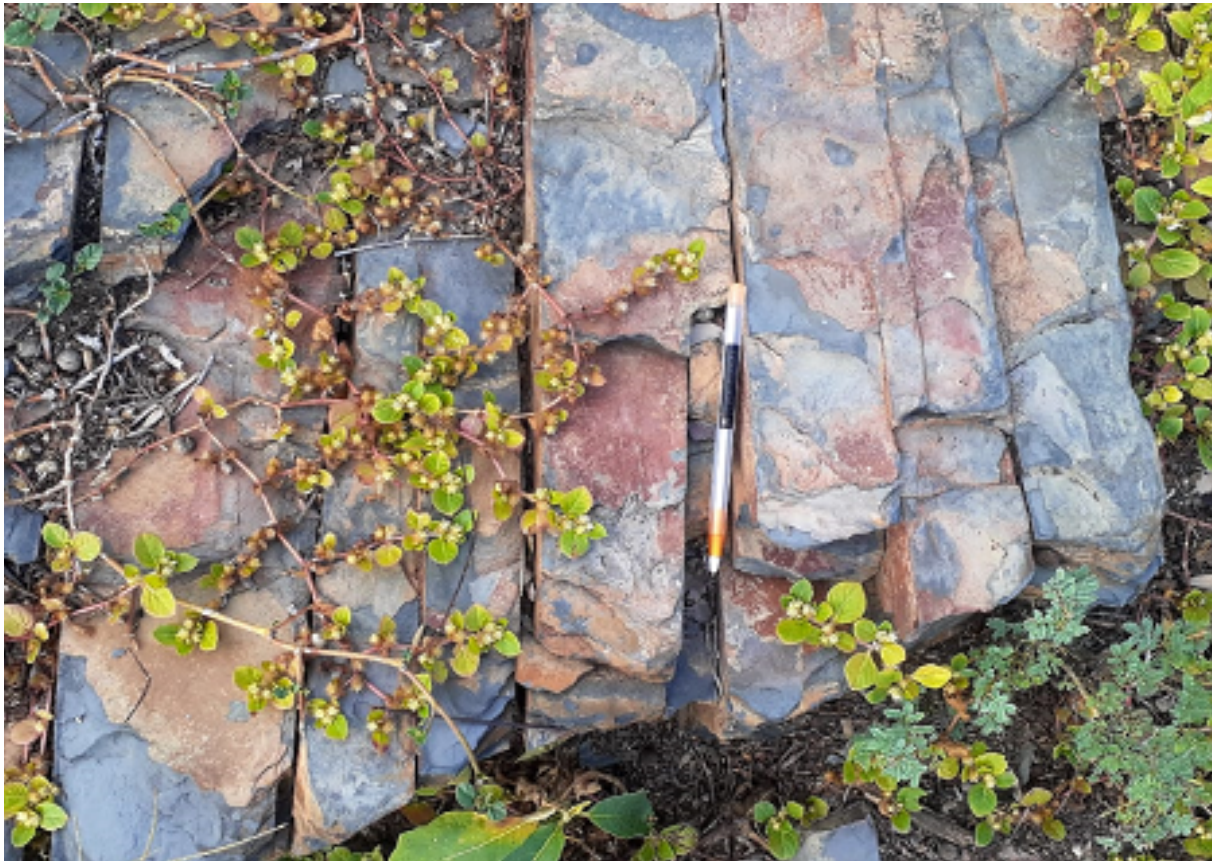
Figure 8: Mogobane Shale deposits, showing an example of a highly fractured Shale which is perfect to be used for cladding.
