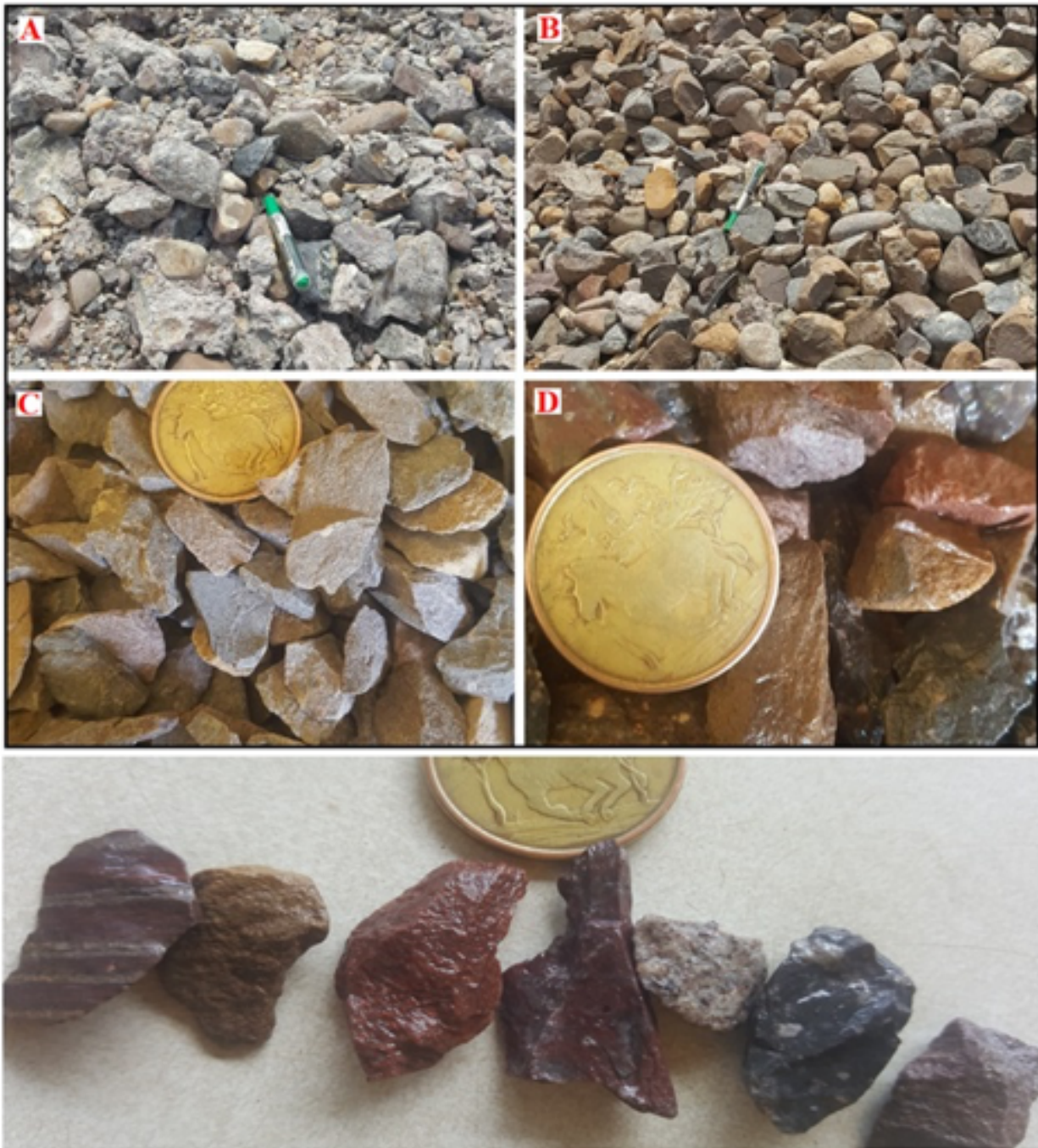
(A) Talpan area composed of fluvial deposits, consisting of boulders and cobbles which were released from their parent rocks by physical weathering and cemented to form conglomerates. B) Talpan re-worked rocks after crushing to remove cementing material C) Dry 19 mm crushed rock D) Wet 19 mm crushed rock
